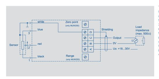
The output signal rises when the actuating rod (LWH) or the actuator (TLH) of the position transducer is moved from 1 to 3 (status on delivery). If the reverse action is required, the terminals 1 (black) and 3 (blue) must be exchanged at the socket insert. After removing the transparent lid, the socket insert can be pushed outwards.
