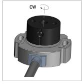
When the marking of the position marker is pointing towards the cable, the sensor output is near the electrical center position (index position).
