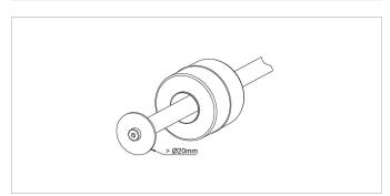
When using floating position markers, we recommend to secure the marker against loss with a washer at the rod end.
