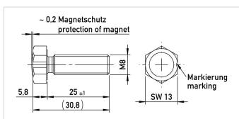
Screw position marker M8 x 25 mm, similar DIN 933/ISO 4017, magnet potted Material Aluminium, anodized
