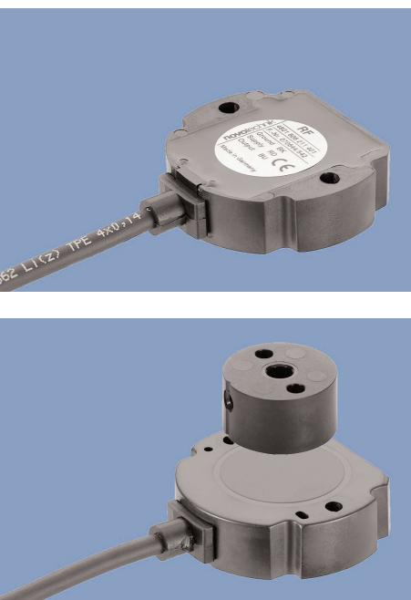
The sensor utilizes the orientation of a magnetic field for the determination of the actual position. Therefore, a magnet is attached to the rotating shaft. The magnetic field orientation is captured with an integrated circuit.
